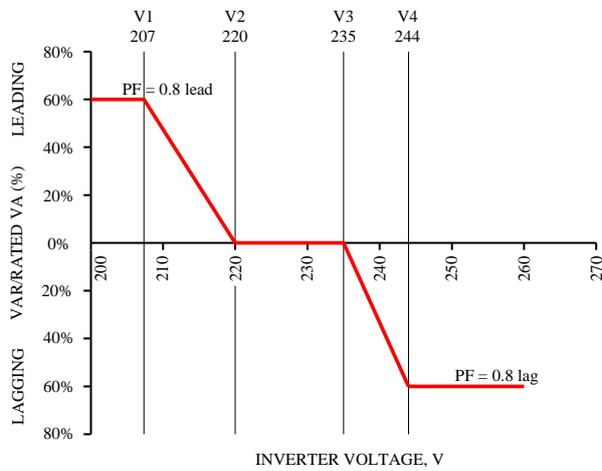
Figure 4. Curve for New Zealand Volt-VAr response mode.
