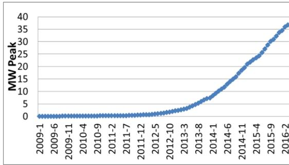
Figure 1. New Zealand photovoltaic (PV) uptake including all capacities: cumulative capacity 2009-2015 (Sources: Data since August 2013 is obtained from [1]. Data prior to this is obtained from [2] and [3]).
