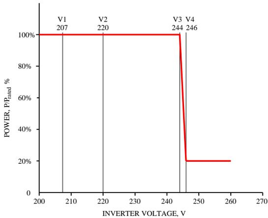
Figure 5. Curve for New Zealand Volt-Watt response mode.
