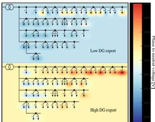
Figure 2. Examples of voltage effects caused by DG power export on a LV network, illustrated by colouring at the points of supply. For the low DG export case, 10% of Installation Control Points (ICPs) are exporting and the network is load dominated. In the high DG export case 100% of ICPs are exporting and significant reverse power flow is occurring causing point of supply over-voltages at the downstream ends of feeders. The background colouring reflects the average network voltage.
