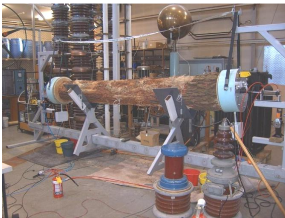
Figure 5. Log test fixture in HV laboratory
